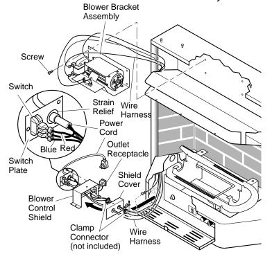
Figure 17 - Installing Blower Bracket Assembly
